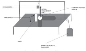
Fig. 1. – Experimental table setup
